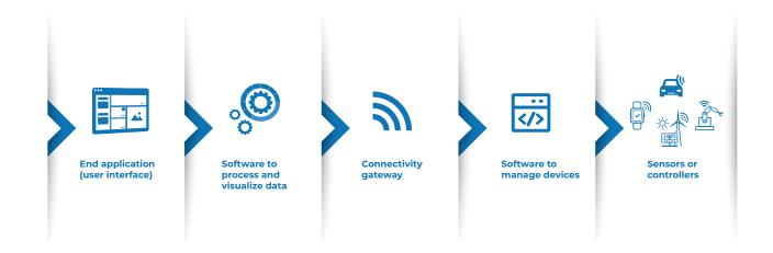
A traditional IoT platform is middleware that provides all of the services and connectivity between the hardware and the applications that need access to the hardware. The specifics of the IoT platform will vary based on the business model but generally speaking there are some major components that are considered fundamental building blocks.
